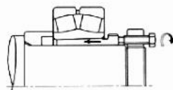
Fig. 14.5 Mounting with Withdrawal Sleeve
