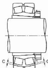
Fig. 14.8 Clearance Measurement of Spherical Roller Bearing
